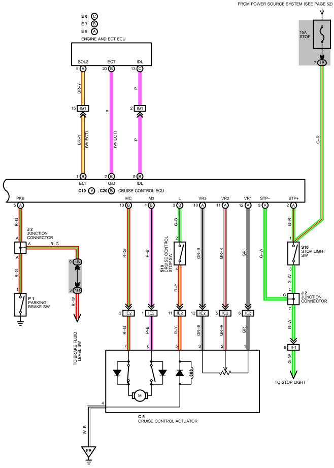
CURRENT IS APPLIED AT ALL TIMES THROUGH STOP FUSE TO **TERMINAL (A) 2** OF THE CONTROL ECU AND **TERMINAL 1** OF STOP LIGHT SWITCH, AND ALSO THROUGH THE DOME FUSE TO TERMINAL (A) 6 OF CRUISE CONTROL ECU.
