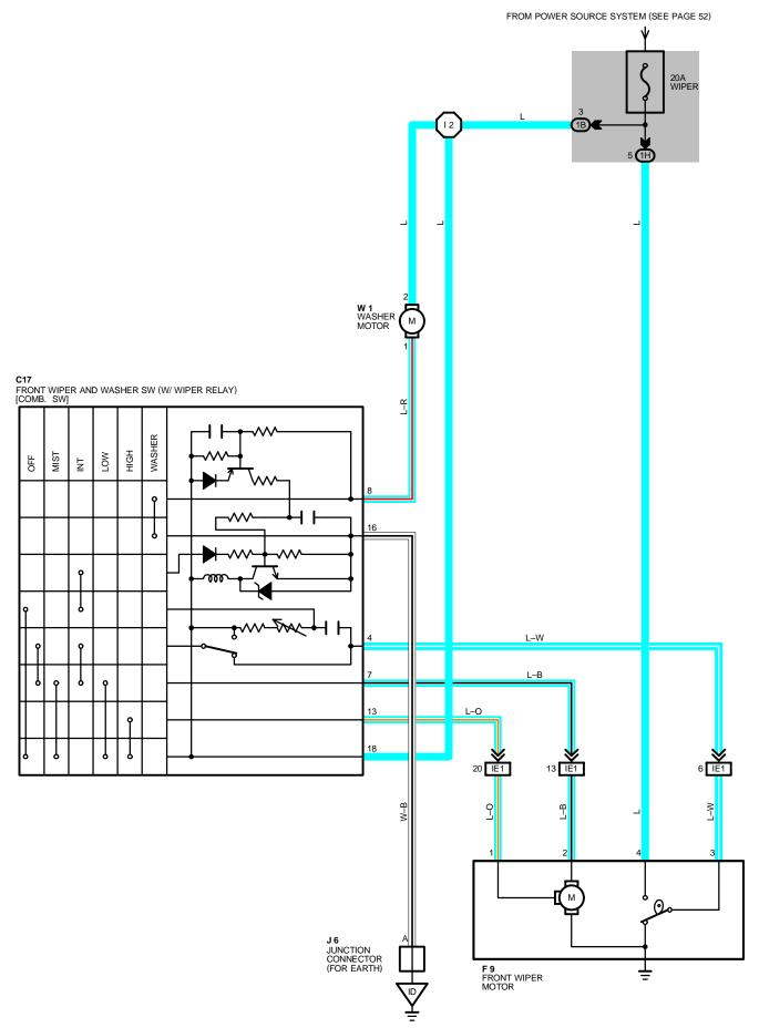
WITH THE IGNITION SW TURNED ON, THE CURRENT FLOWS TO **TERMINAL 18** OF THE WIPER AND WASHER SW, **TERMINAL 2** OF THE WASHER MOTOR AND **TERMINAL 4** OF THE FRONT WIPER MOTOR THROUGH THE WIPER FUSE.
