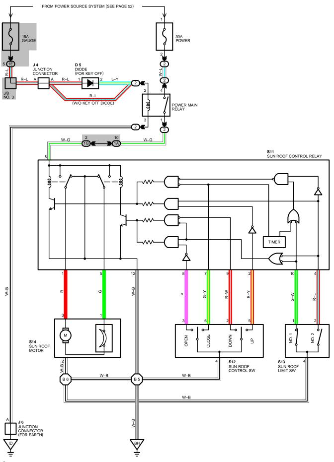
CURRENT ALWAYS FLOWS TO **TERMINAL 4** OF THE POWER MAIN RELAY THROUGH THE POWER FUSE, WITH THE IGNITION SW TURNED ON, CURRENT FLOWS THROUGH THE GAUGE FUSE TO **TERMINAL 2** OF THE POWER MAIN RELAY. THIS ACTIVATES THE RELAY AND CURRENT FLOWING TO **TERMINAL 4** OF THE POWER MAIN RELAY FLOWS TO **TERMINAL 1** OF THE POWER MAIN RELAY  $\rightarrow$  TO **TERMINAL 6** OF THE SUN ROOF CONTROL RELAY.
