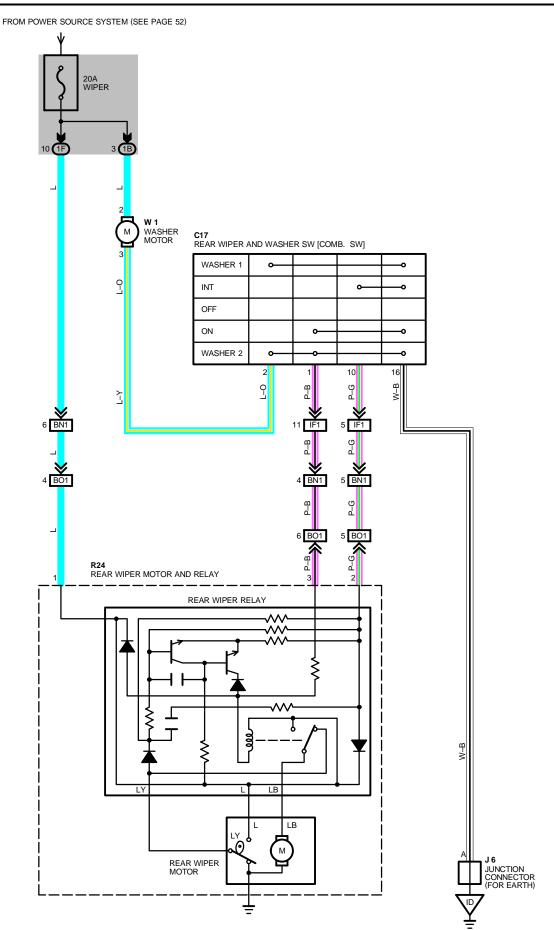
WHEN THE IGNITION SW IS TURNED ON, CURRENT FLOWS TO **TERMINAL 2** OF THE REAR WASHER MOTOR, **TERMINAL 1** OF THE REAR WIPER MOTOR AND RELAY THROUGH THE WIPER FUSE.
