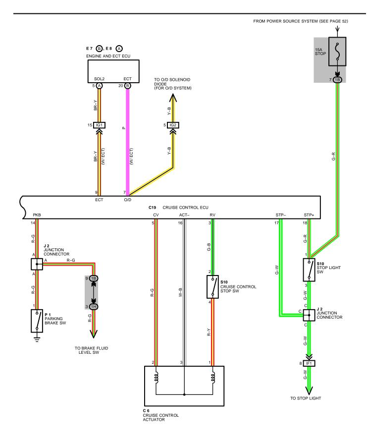
CURRENT IS APPLIED AT ALL TIMES THROUGH STOP FUSE TO **TERMINAL 18** OF THE CRUISE CONTROL ECU AND **TERMINAL 1** OF THE STOP LIGHT SW.
