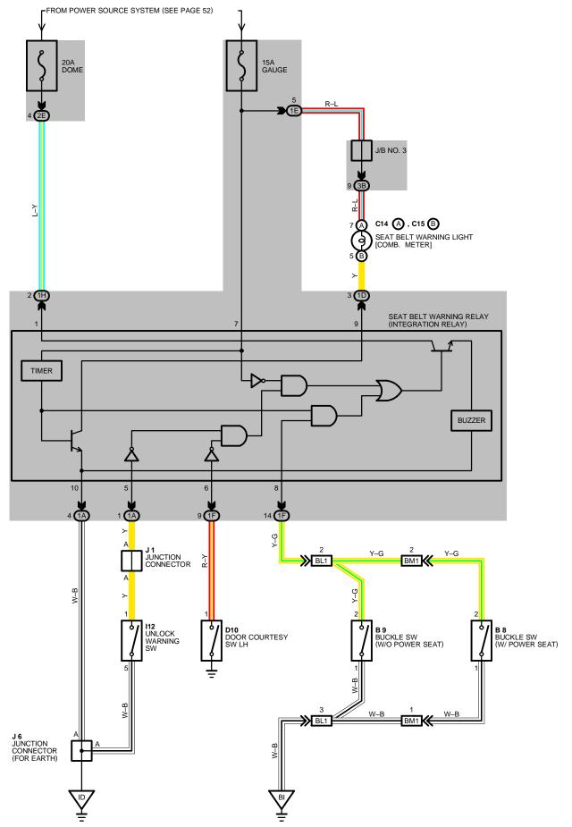
CURRENT ALWAYS FLOWS TO **TERMINAL 1** OF THE SEAT BELT WARNING RELAY (INTEGRATION RELAY NO.1) THROUGH DOME FUSE.
