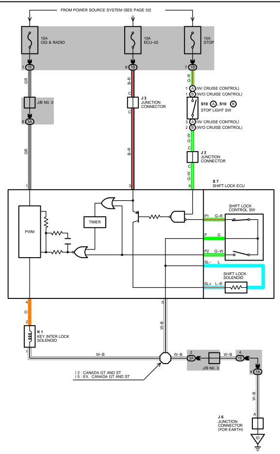
WHEN THE IGNITION SW IS TURNED TO ACC POSITION THE CURRENT FROM THE CIG FUSE FLOWS TO TERMINAL 1 OF THE SHIFT LOCK ECU. IN THE ON POSITION. THE CURRENT FROM THE ECU-IG FUSE FLOWS TO TERMINAL 3 OF THE ECU.
